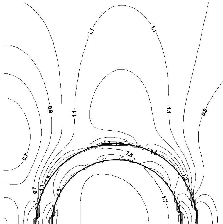
Fig. 8. Contours of (\sigma_1 - \sigma_2)/\sigma_0 for two inclusions with stiff coatings.
